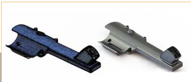
Scan of the gearbox (L) and a 3D render of the finished casting (R)
